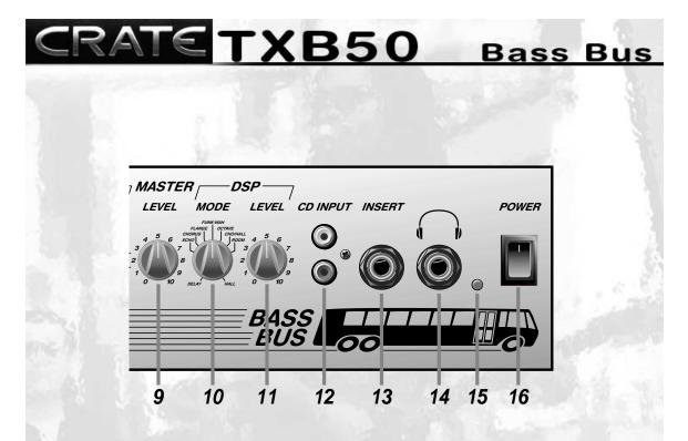
9. MASTER LEVEL: Use this control to adjust the overall output of the amplifier.
